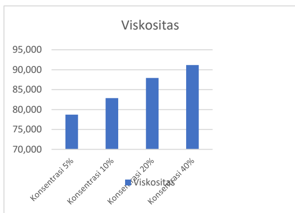
Picture 2 Results of Viscosity Test Preparation of Giant Ginger Extract Toothpaste Using Brookfield Viscosity at RPM 50 Spindle No.64
