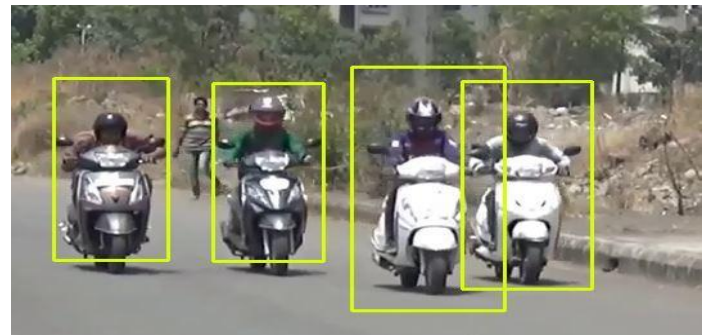
Fig.7: Vehicle (Bike) Detection by LVC & Haar Cascade
