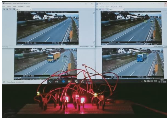
Fig. 20: Detection of cars in first,third,fourth video-frame (green in first and fourth) as total number of cars in first and fourth is more
