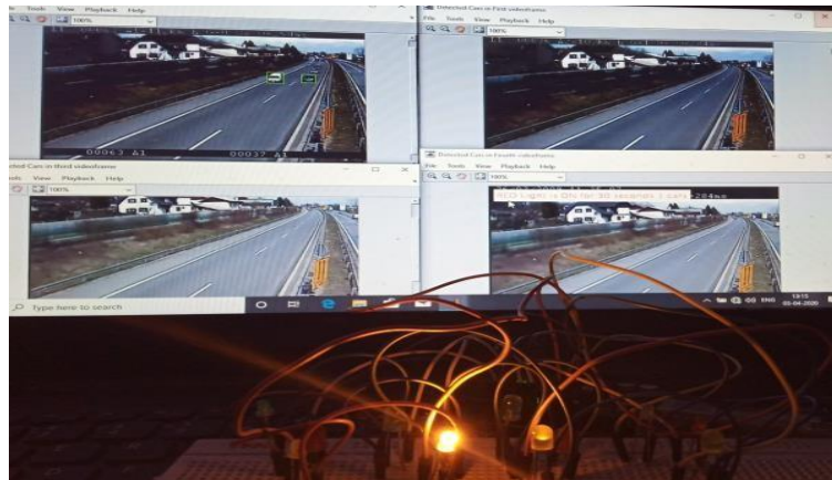
Fig. 17: Detection of cars in second video-frame (second road) only and corresponding output (Red in first and fourth road and Green in second and third)
