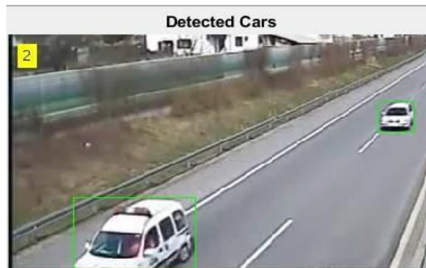
Fig. 16: Detection of cars in fourth video-frame (fourth road)
