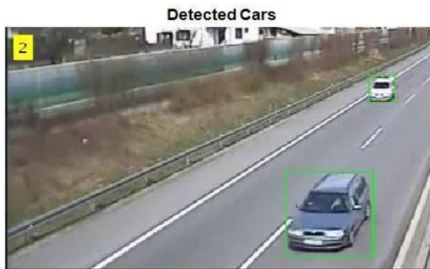
Fig. 14: Detection of cars in second video-frame (second road)
