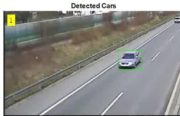
Fig. 15: Detection of cars in third video-frame (third road)
