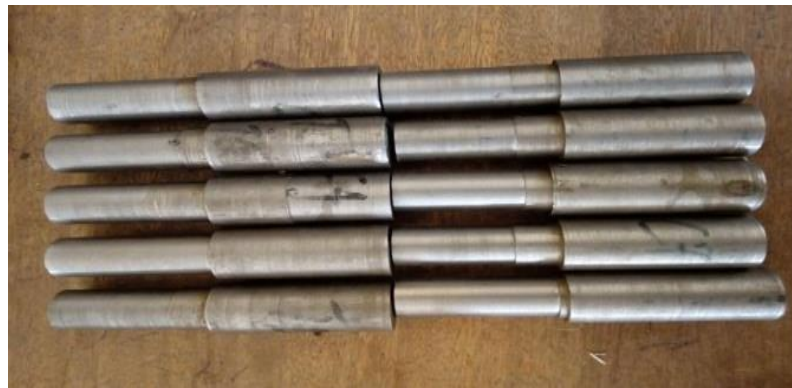
Plate 1: Stepped Turned mild steel workpiece.
