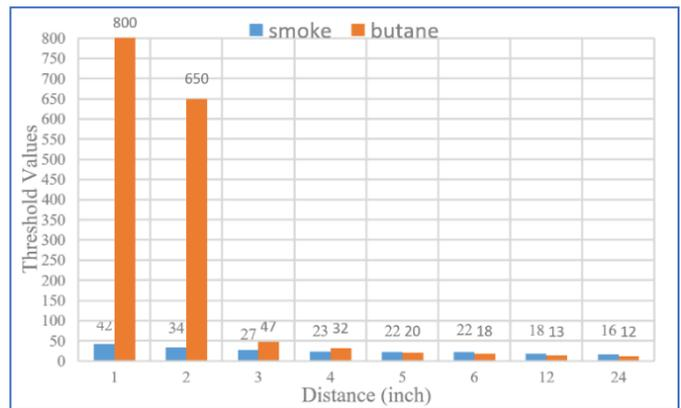
Fig.7: Butane Sensor Test Results
