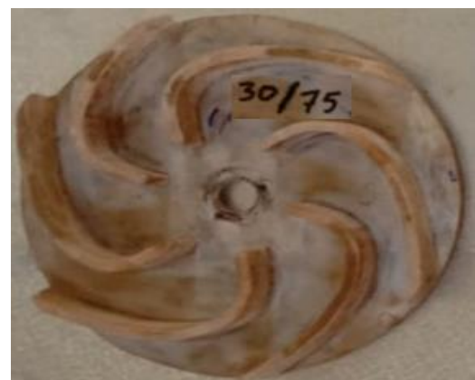
Fig 2:- Impeller with variations in the angle of entry and exit angle of 30/75
