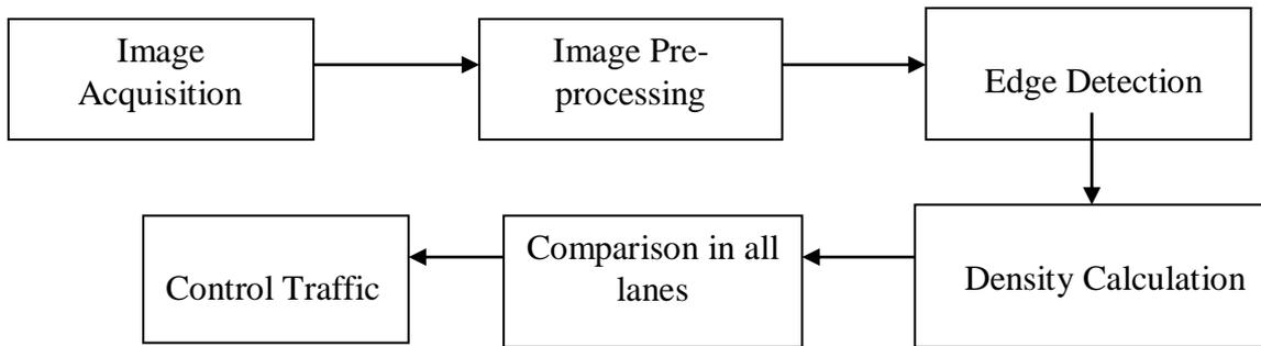
Fig. 1: General Framework for Traffic Control System using Image Processing
