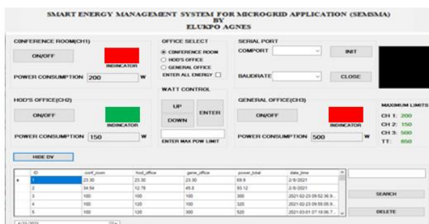
Fig. 5: HOD’s office ON while Conference room and Secretary’s (general office) OFF
