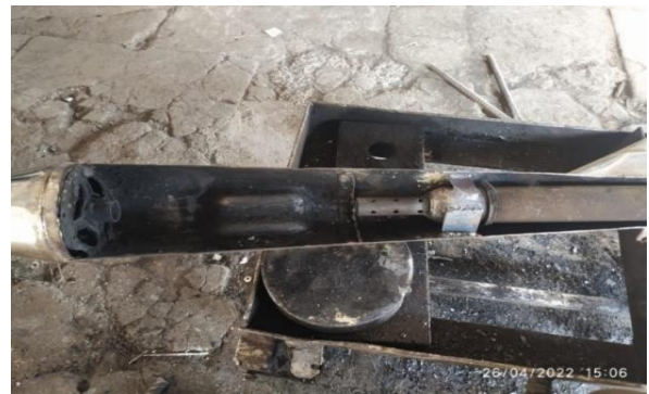
Fig.10. Silencer after cutting the components
