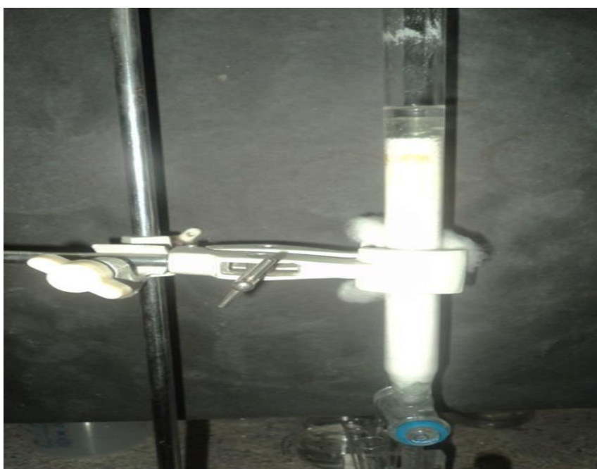
Fig. 2: Purification of Tylophora indica alkaloids using Column chromatography.
