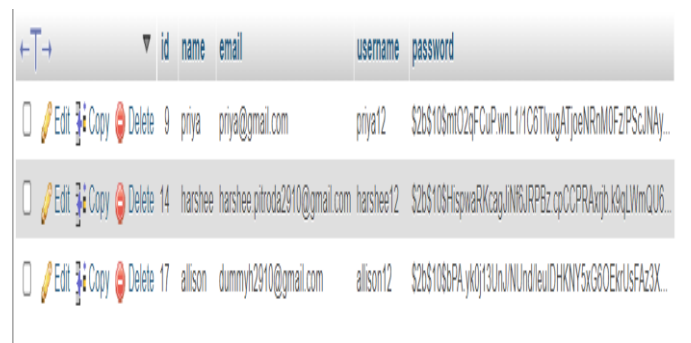
Fig. 78: User database and a snippet of the password being salt hashed and stored
