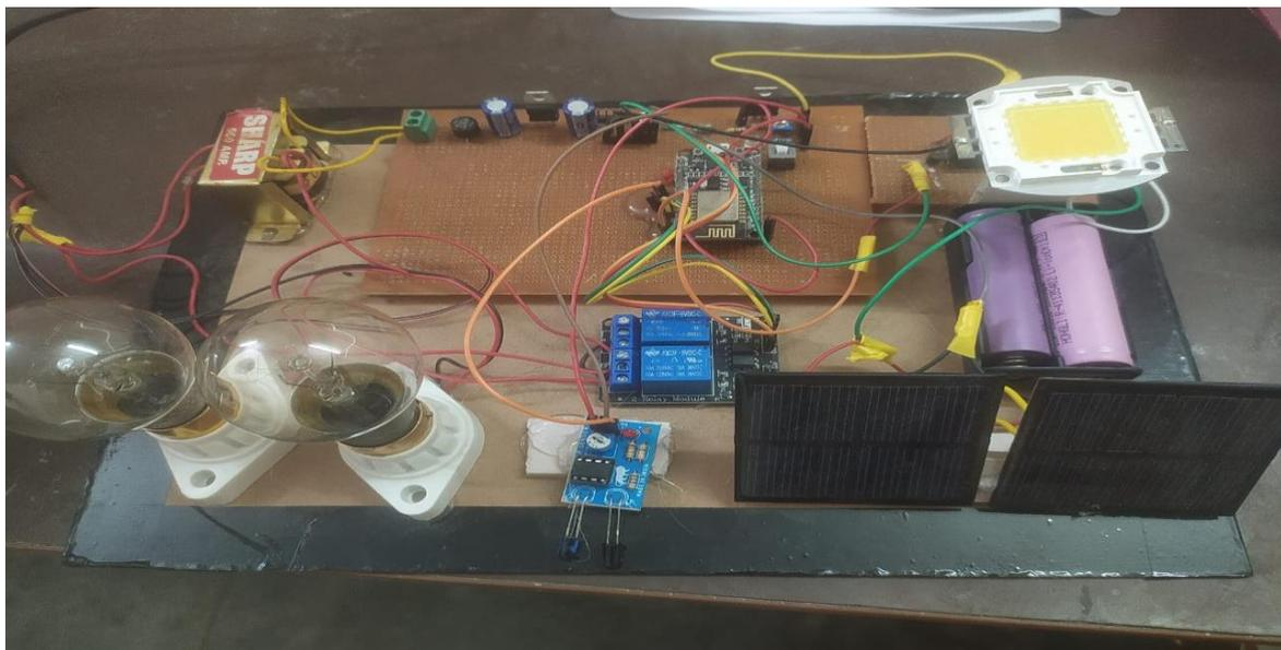
Fig. 1: An IoT based energy management system
