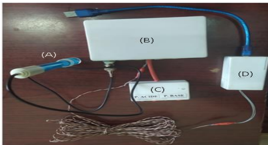
Fig. 8: Overall view of a continuous or on-line pH acquisition system
