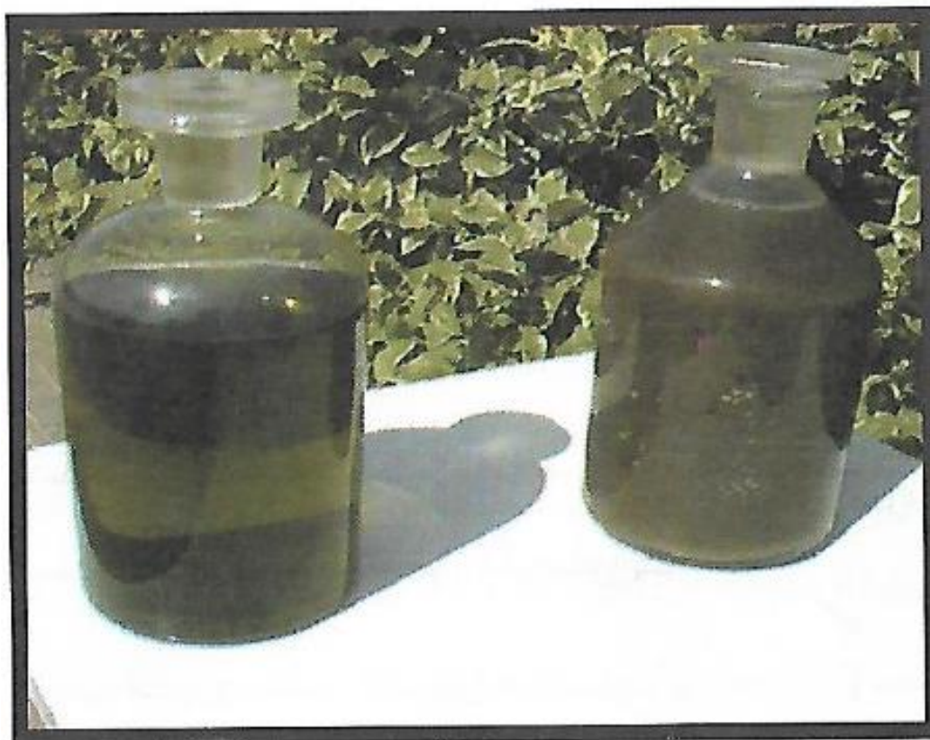
Fig. 6: Local phosphoric acid before and after treatment
