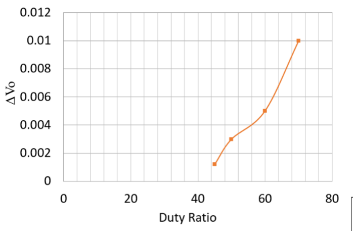
Fig. 11: Output Voltage Ripple Vs Duty Ratio
