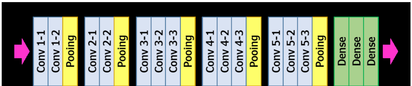
Fig 5:- VGG16 layered architecture
