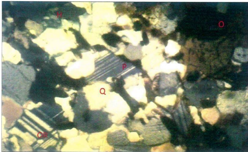
Plate 7: Photomicrograph of granite gneiss under cross polarized light (x 10) B=Biotite, H=Hornblende, O= Opaque, Or= Orthoclase, M= Muscovite, Q= Quartz,P= Plagioclase.
