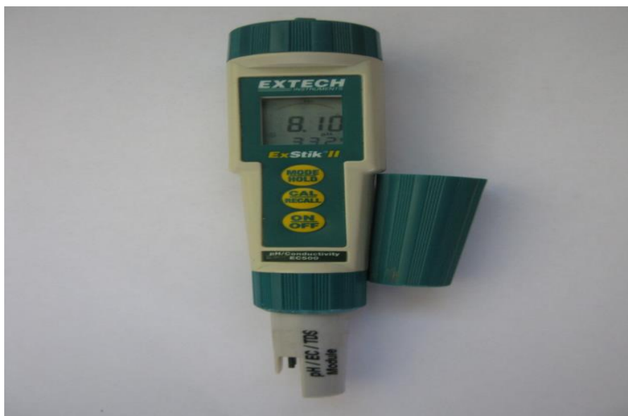
Fig. 5: pH-TDS-salinity meter EXTECH Instruments ExStik II EC 500
