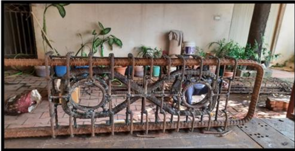
FIG 16: CONNECTION CAGE WITH INFINITY RING.
