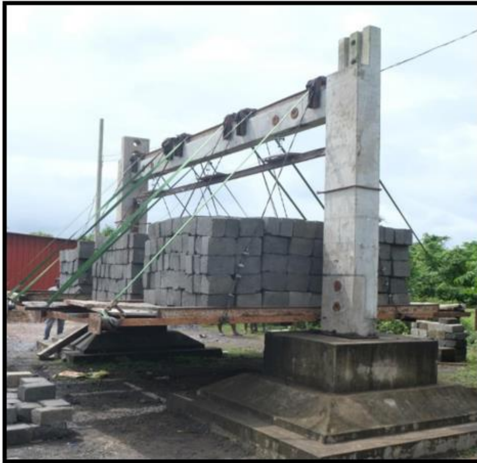
FIG 55: FULLY LOADED SUSPENDED PLATFORM.- SIDE VIEW
