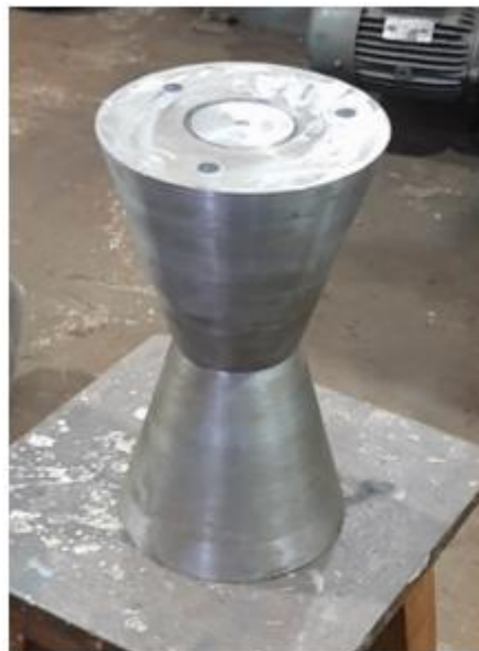
FIG 11: PICTURE OF ASSEMBLED PIN (THREADED BOLT) & CONICAL NUTS
