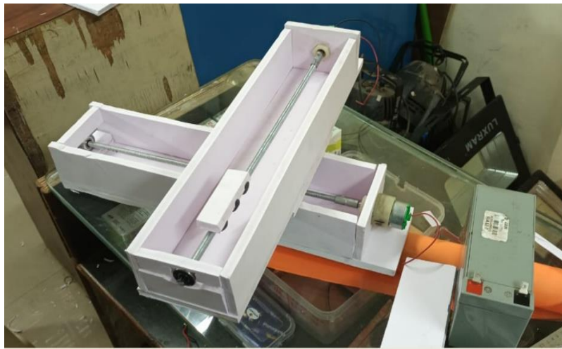
Fig 4:- Experimental setup of automatic PCB track design machine.
