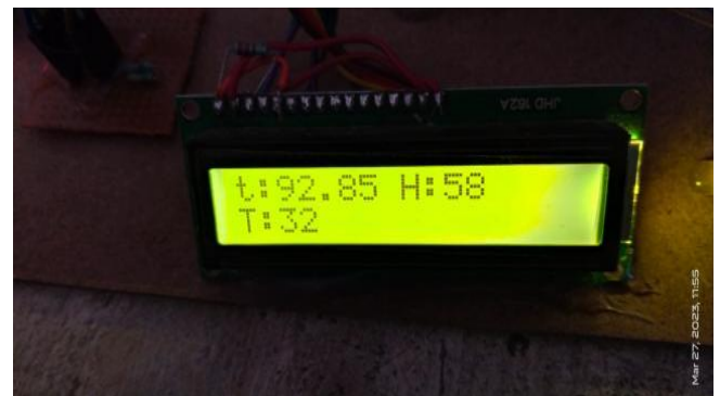
Fig 7 Temperature and Heartbeat verification
