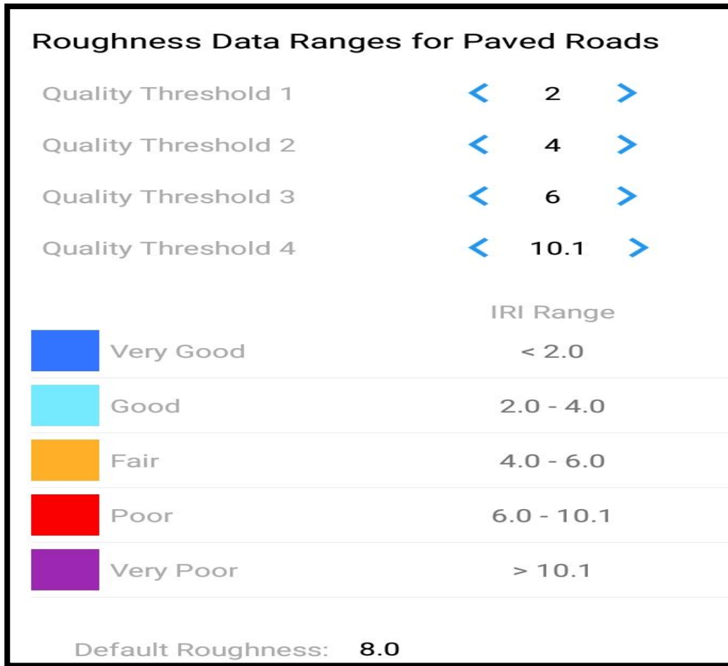
Fig. 3: Roughness Data Ranges ForPaved Roads
