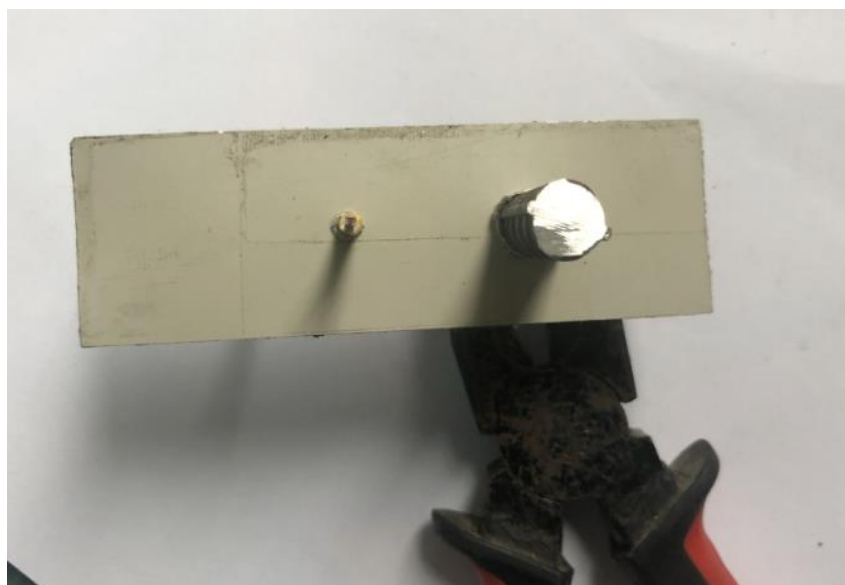
Fig. 5: The cutting surface of the electrode rod
