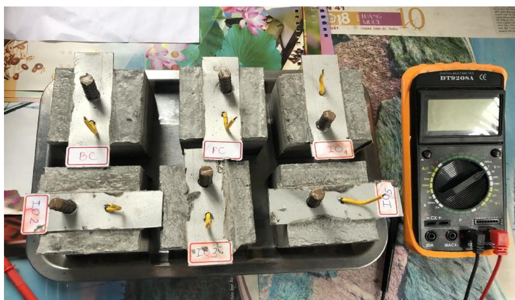
Fig. 7: Measuring the corrosion potential
