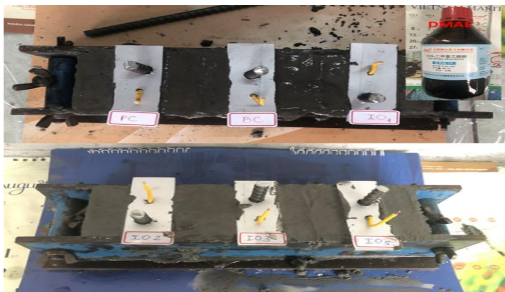
Fig. 6: Samples molded in 70.7mm cell formwork
