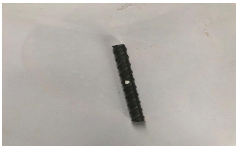
Fig. 2: CB300-V rebar cut as the sample electrode
