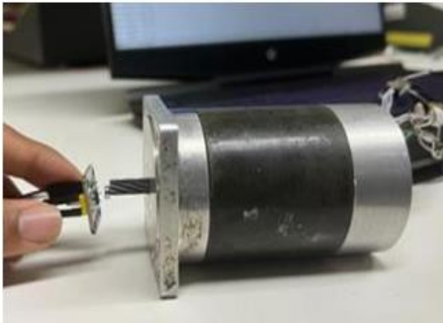
Fig 5 AS5600 Brought Close to the Magnet Placed on the Rotor of SRM
