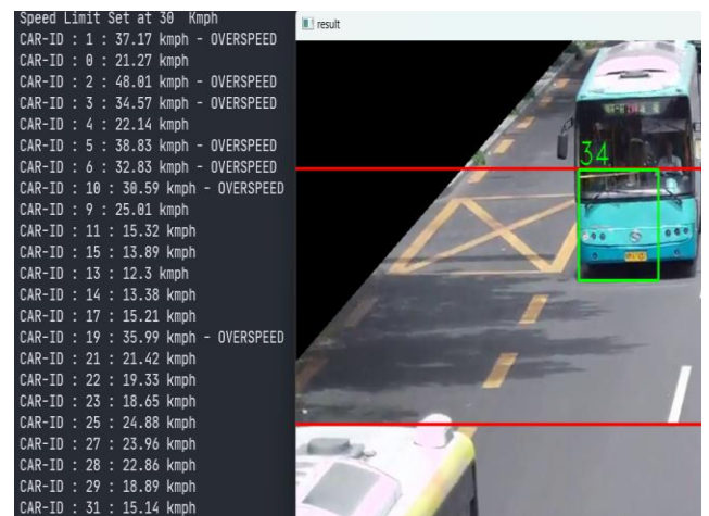
Fig 9 Speed Estimation with Speed Limit 30kmph
