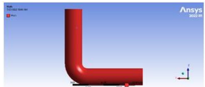
Fig 1 Pipe Geometry and Boundary Condition
