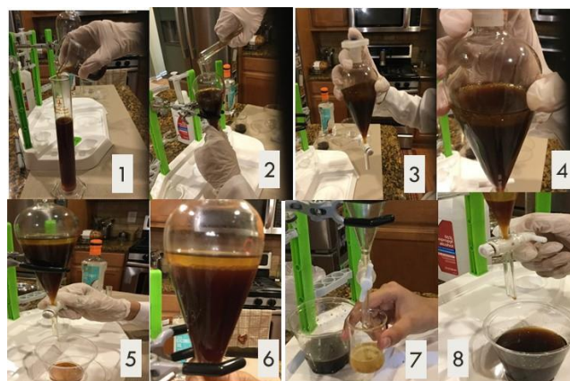
Fig. 4. Scaled-up extraction of oil from Spent Ground Extracts. 1-3: Addition of hexane to washed saponified oil in separating funnel; 4-6: Shaking after addition of saturated
