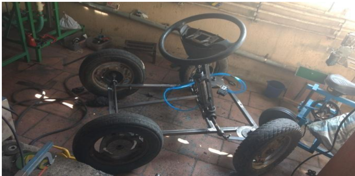
Fig 6 Assembly of Collapsible Steering Wheel to Chassis
