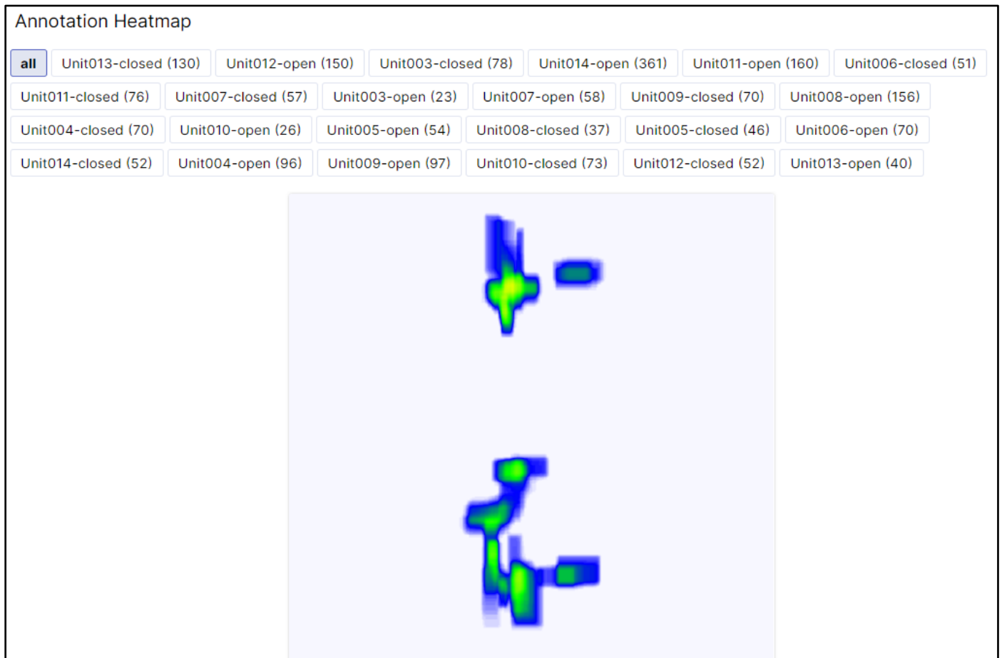
Fig 20 Annotation Heatmap, Providing a Visual Representation of the Density of Object Annotations within Images
