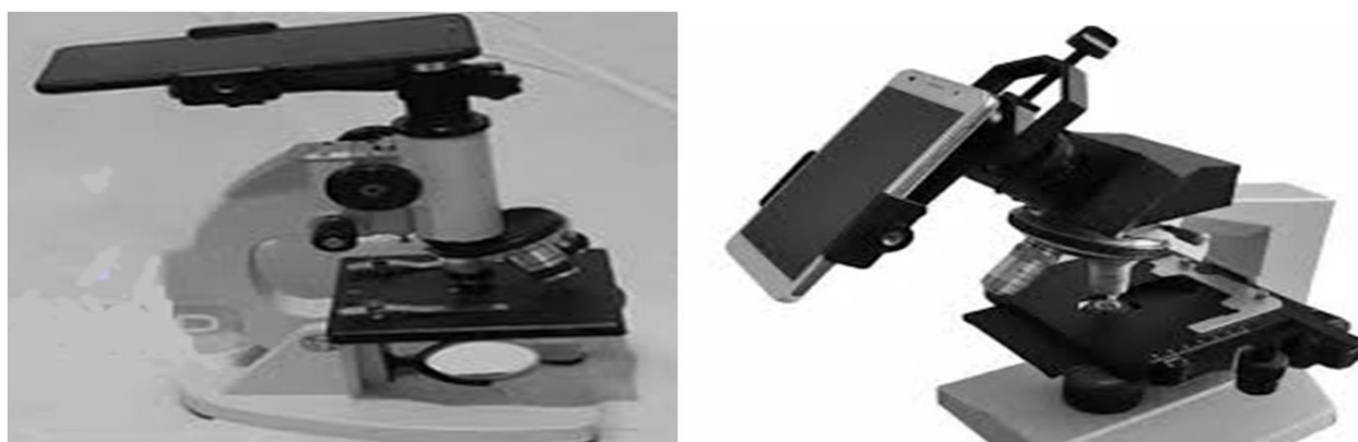
Fig 4 Adding a Cellphone above the Eyepiece Lens, Part of the Microscope.
