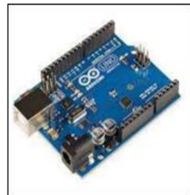
Fig 3 Acts as the Central Processing Unit for Interpreting IR Signals and Controlling the Servo Motor
