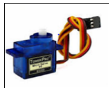
Fig 4 Output Actuator Responsible for Physical Rotation to the Specified Angle.
