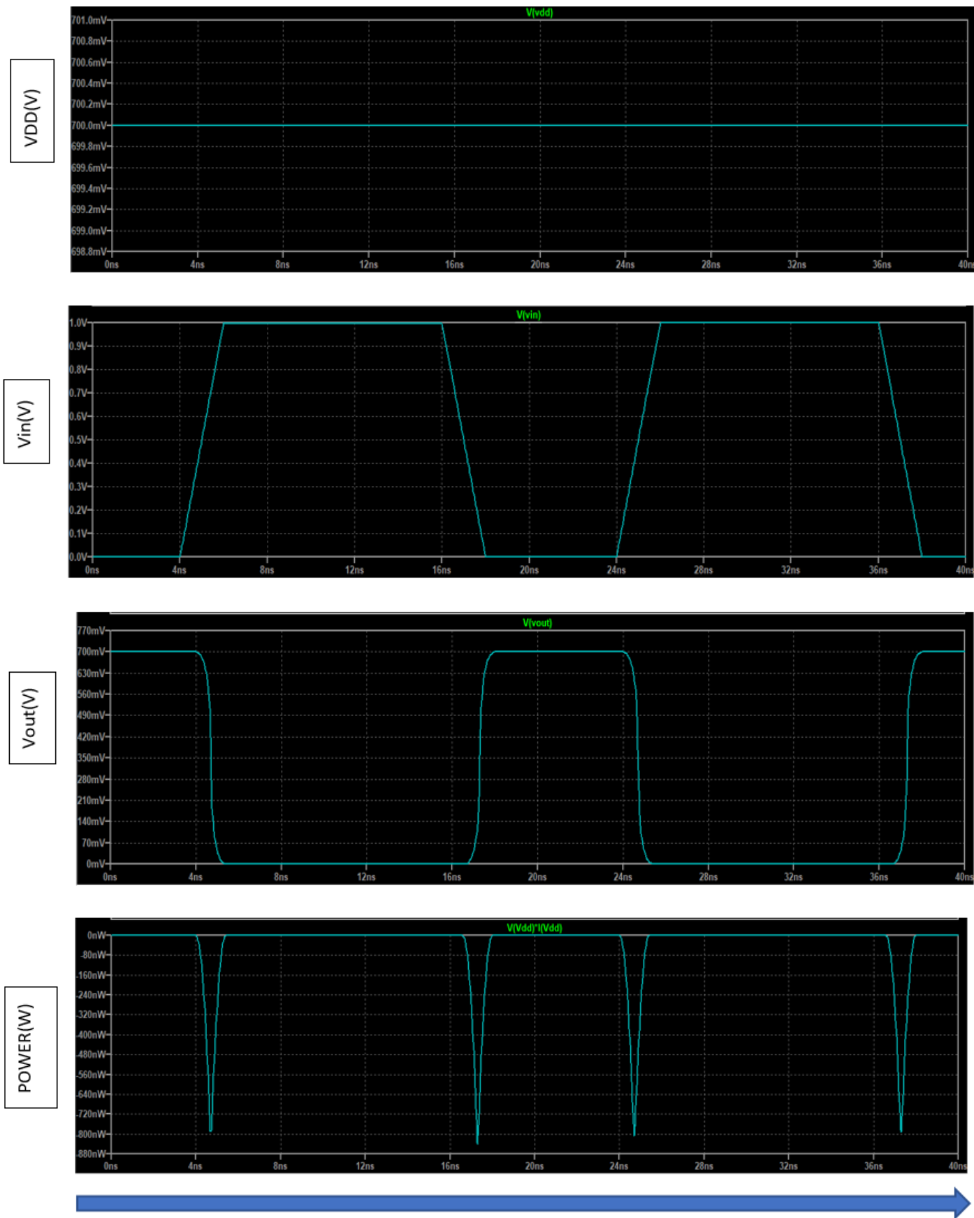
Time scale of 0-40ns Fig 4. Inverter based on MoS 2 transistor. Vdd, Vin, Vout, power.
