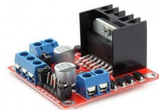
Fig.8. L298N H Bridge motor driver board
