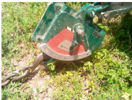
Plate 1; the dynamometer Plate 2; dynamometer coupled for tractor trace method of draught measurement and Plate 3; draught measurement for disc plough using tractor trace technique
