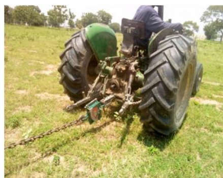
Plate 1; the dynamometer Plate 2; dynamometer coupled for tractor trace method of draught measurement and Plate 3; draught measurement for disc plough using tractor trace technique
