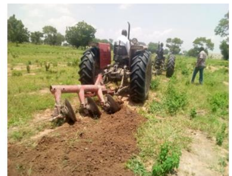
Plate 1; the dynamometer Plate 2; dynamometer coupled for tractor trace method of draught measurement and Plate 3; draught measurement for disc plough using tractor trace technique
