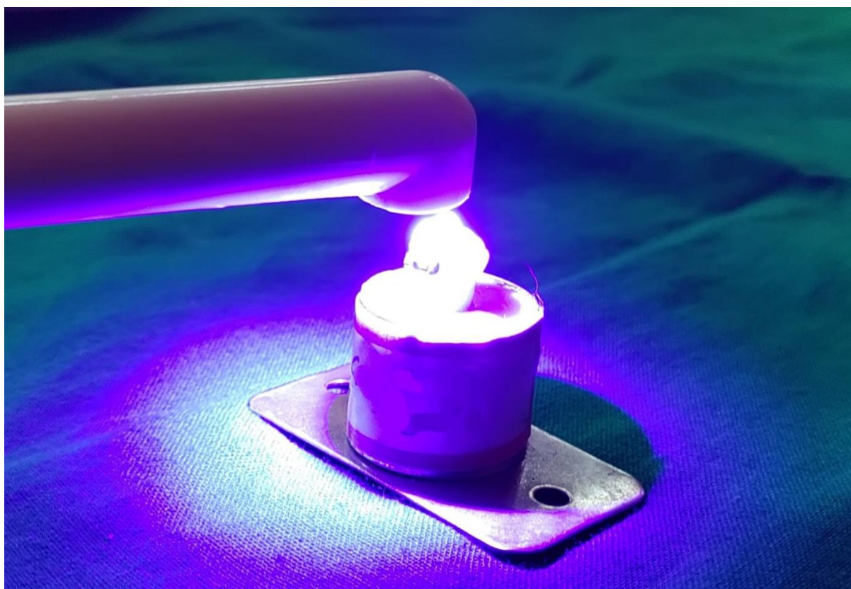
Fig. 7: Curing of Adhesive
