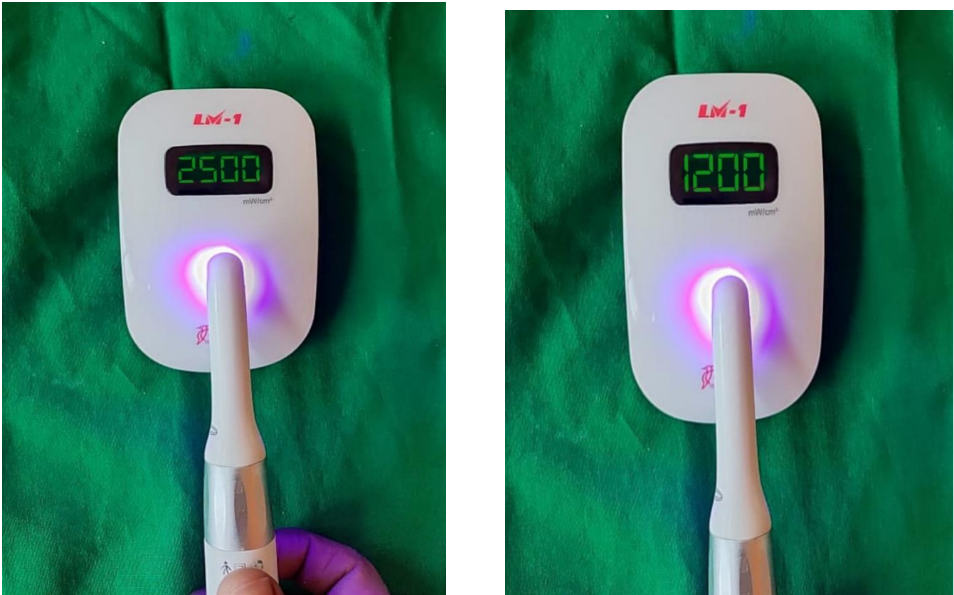
Fig. 8: LED Curing Light capable of producing different intensities of light
