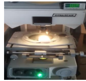
Fig 12. Profile projector for measurement of interimplant distance
