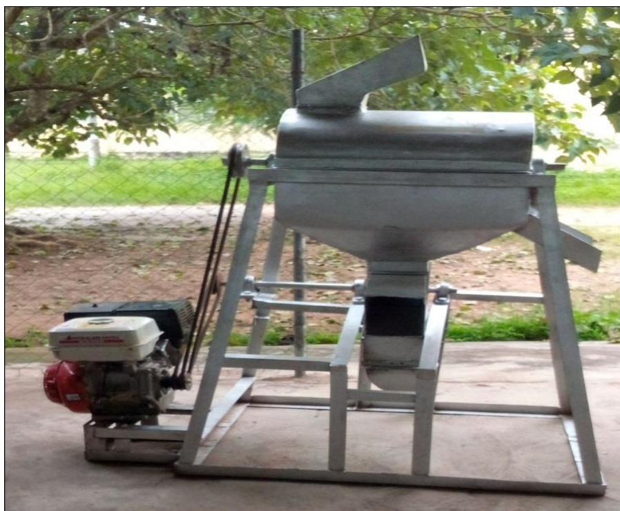
Fig 2 The Combined Shelling and Winnowing machine
