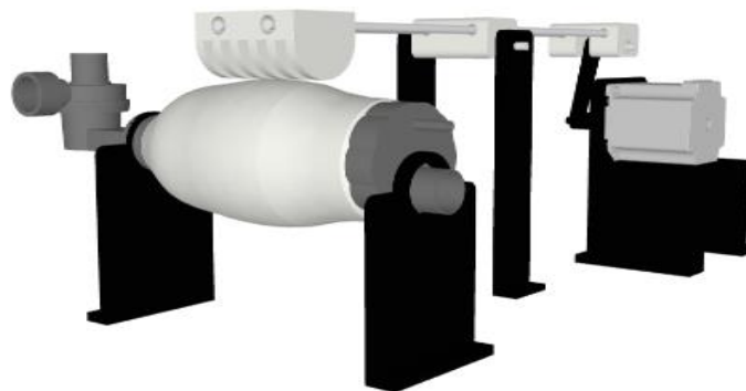
Fig. 2: Design of portable ventilator
