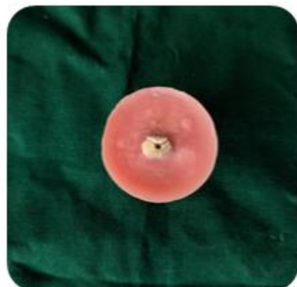
Fig 5 Prepared Sample after Testing Under UTM
