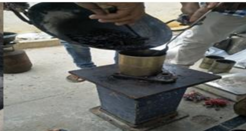
Fig 4 Placing of Aggregates and Bitumen in The Mould After Mixing
