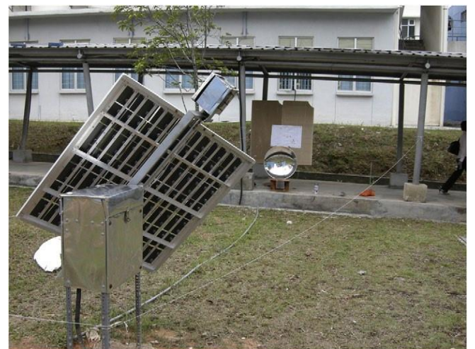
Fig. 2. The prototype of novel solar furnace system consisted of the fixed geometry NIFH heliostat and the secondary parabolic concentrator in the campus of Universiti Tunku Abdul Rahman.
