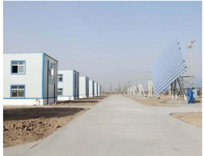
Fig. 1. A 6 X 6 m working prototype of the new solar furnace using nonimaging focusing heliostat constructed in NingXia province, PR China.
