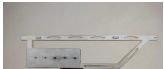
Fig 9 .3D printed Fuselage with ABS material .
