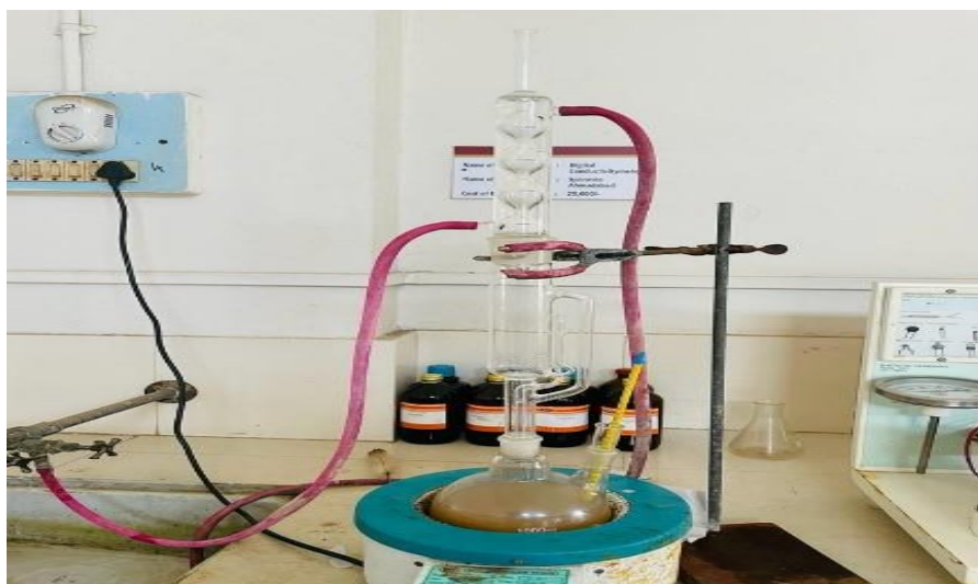
Fig. 1: Experimental setup of Extraction
