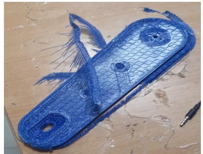
Fig 6 Damaged Part During Printing
