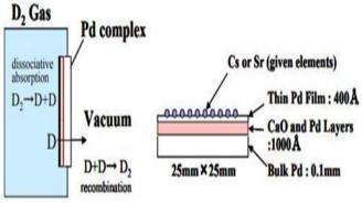
Fig 8 Transmutation Experimental Setting in ref [8]
