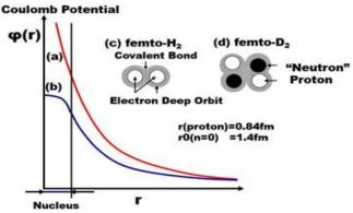
Fig 5 Electron deep orbit based on (b) the correct coulomb potential with the comparison of (a) point charge coulomb potential.(c) femto  $D_2$ , (d) femto  $H_2$
