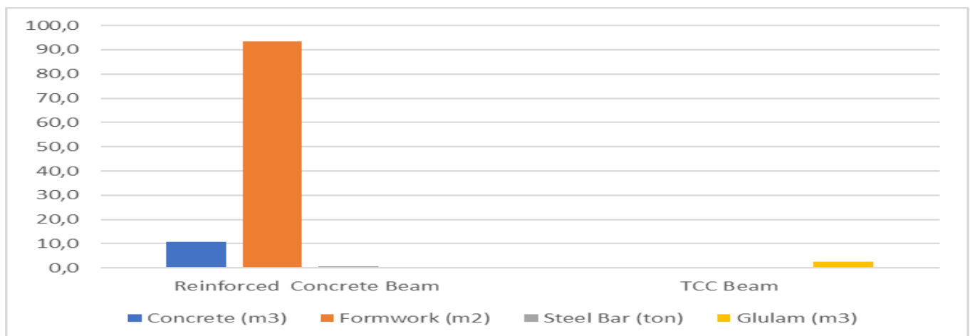
Fig 5 Comparison between TCC Beam and RC Beams in Terms of Concrete Volume, Formwork, Steel Bar, and Volume of Timber
