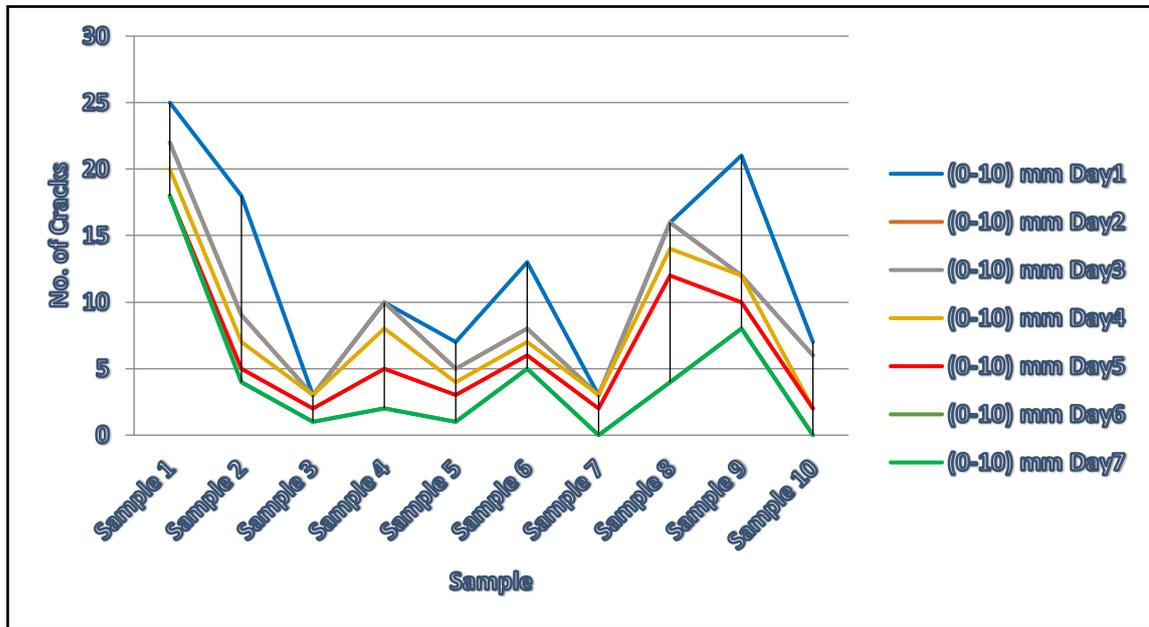
Fig. 5: Showing the number of cracks propagated in (0-10) mm soil samples per week
