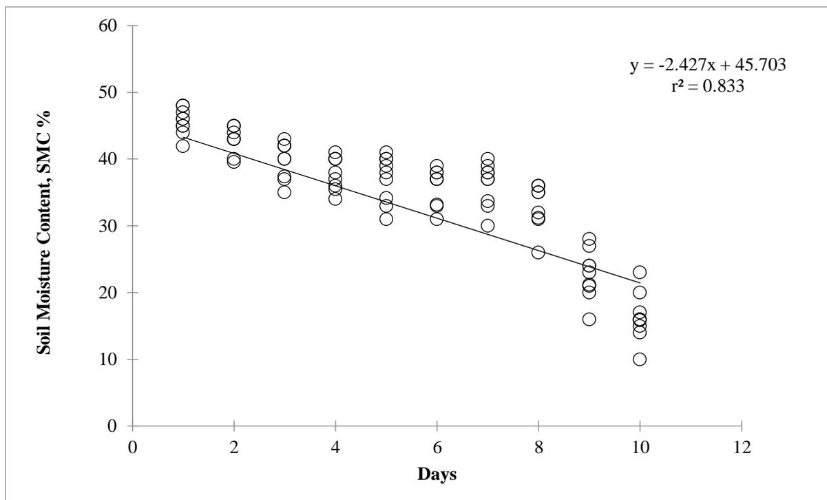
Fig. 2: Relationship in Soil Moisture Contents of different vertisol soil samples in ten days
