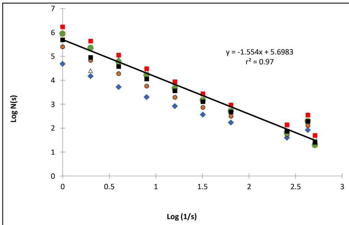
Fig. 4: Relationship between log (1/s) and log N(s) of sample 2 of a Black Cotton soil (Vertisol)
