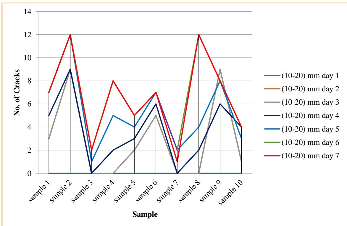
Fig. 6: Showing the number of cracks propagated in (10-20) mm soil samples per week
