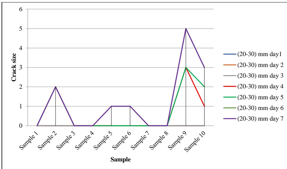
Fig. 7: Showing the number of cracks propagated in (20-30) mm soil samples per week
