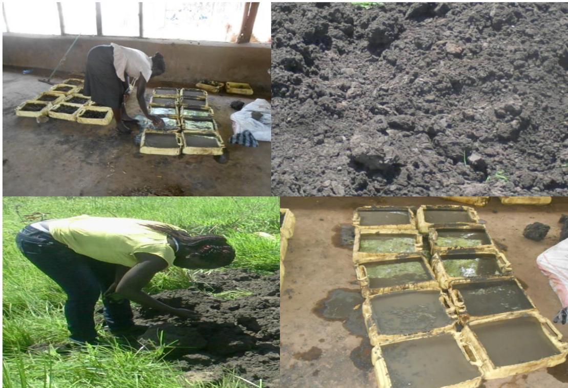
Plate 1: Preparation of vertisol soils for an Experiment to determine cracks properties
