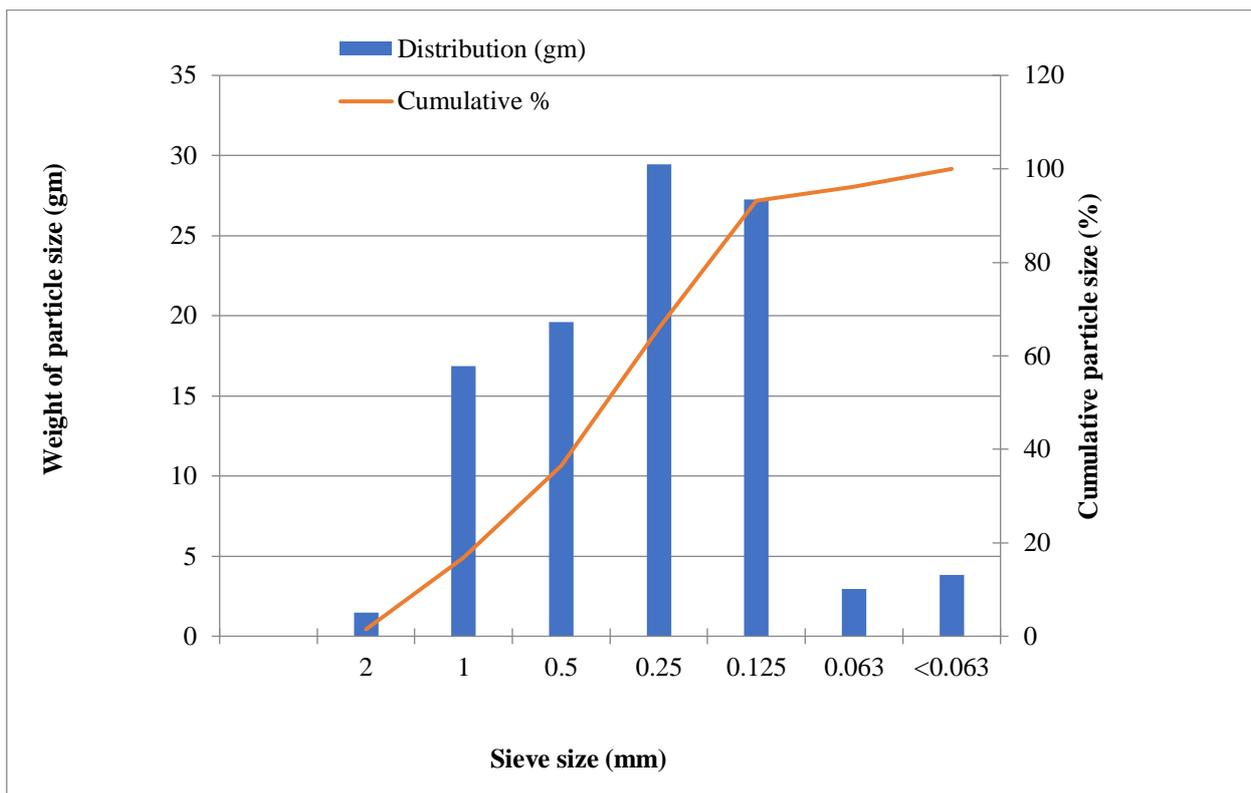
Fig. 1: Particle size distribution of a selected vertisol soil sample
