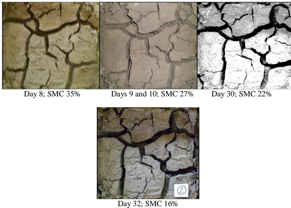
Fig. 3: Sequences of crack development and propagation behavior in soil sample 2 of a remolded vertisol
