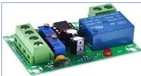
Fig. 9: Power control module
