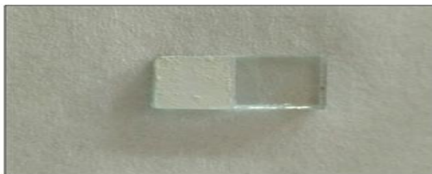
Fig. 2: ZnO/FTO electrodes produced in the electrodeposition process
