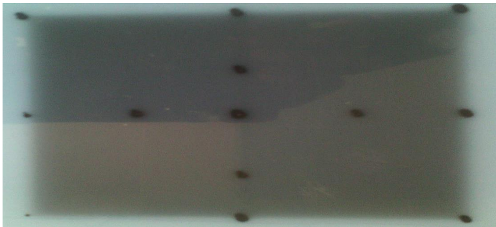
Fig. 8: Congruency between Radiation and Optical Field (10 × 10 cm 2 )
